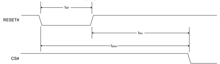
Figure 17 - Hardware Reset Timing Diagram
