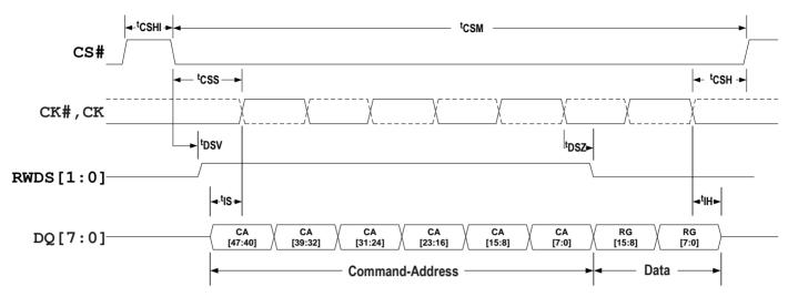
Figure 26 - Write Operation without Initial Latency (Register Write)
