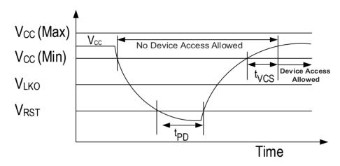
Figure 16 - Power Down or Voltage Drop
