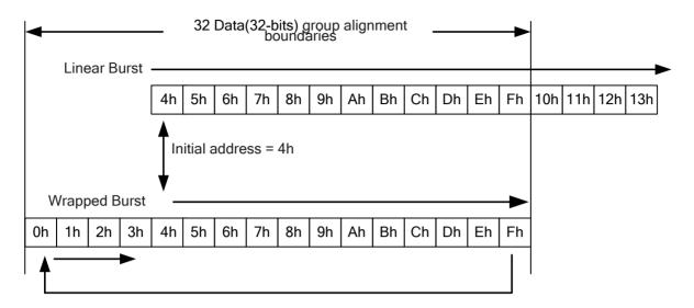
Figure 2 - Linear Versus Wrapped Burst Sequence
