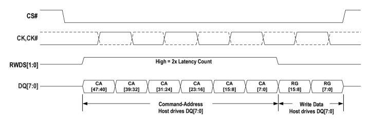
Figure 8 - Write Operation without Initial Latency (Register Write)
