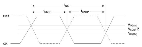
Figure 22 - Clock Characteristics
