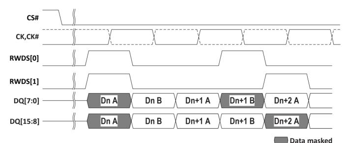
Figure 5 - Data Placement during a Write Transaction
