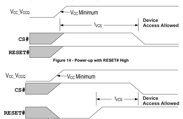
Figure 15 - Power-up with RESET# Low
