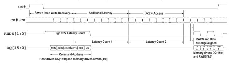
Figure 6 - Read Transaction with Additional Initial Latency
