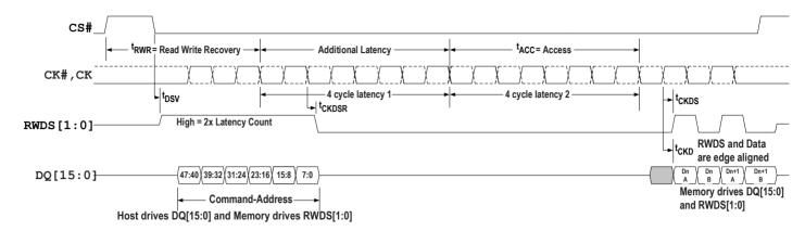
Figure 23 - Read Timing Diagram — With Additional Latency
