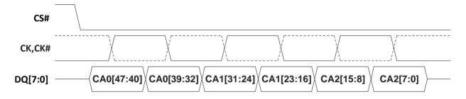
Figure 3 - Command-Address (CA) Sequence
