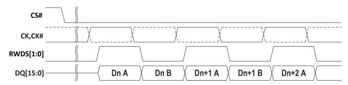
Figure 4 - Data Placement during a Read Transaction
