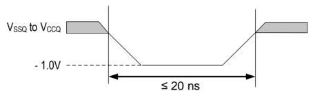
Figure 18 - Maximum Negative Overshoot Waveform
