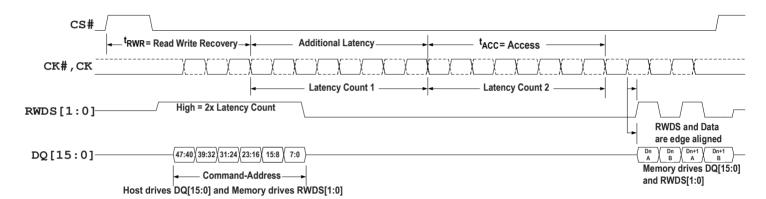
Figure 1 - Read Transaction, Additional Latency Count
