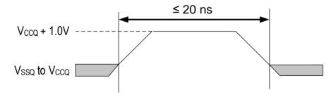
Figure 19 - Maximum Positive Overshoot Waveform
