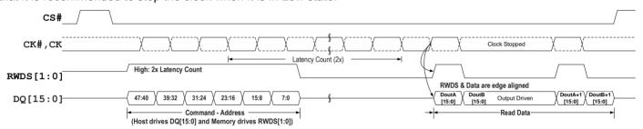
Figure 9 - Active Clock Stop during Read Transaction (DDR)
